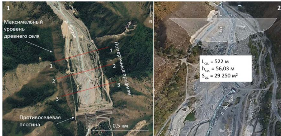
Figure 8 – The section of the Talgar River valley where the giant ancient mudflow exited the valley. The marked features include the maximum flow level on the valley slopes, cross-sectional profiles, averaged cross-section, and an 8.5 million m 3 mudflow protection dam constructed in 2005 [10]
